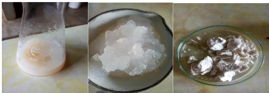
Figure 22. (a)Precipitated Silica after Addition of 2.5M H 2 SO 4 (B) Silica Gel after Filtration(C) Silica after Drying
