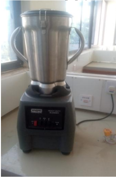
Appendix 2: Heavy duty blender that was used for grinding the leaves and root of C.papaya
