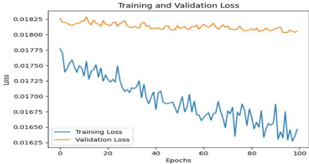
Figure 4.7: Softmax activation function training loss.
