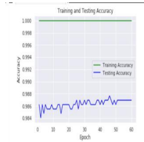
Fig. 28. Training and Testing Accuracy for ConvNet using Learning Rate of 0.0001 with 10 Disease Classes.
