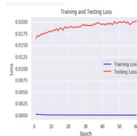
Fig. 29. Training and Testing loss for ConvNet using Learning Rate of 0.0001 with 10 Disease Classes.
