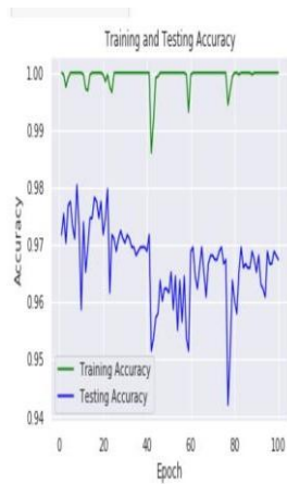
Fig. 44. Training and Testing Accuracy for ConvNet using Learning Rate of 0.00001 with 16 Disease Classes.
