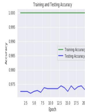
Fig. 42. Training and Testing Accuracy for CNN using Learning Rate of 0.00001 with 16 Disease Classes.
