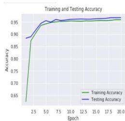
Fig. 6. Training and Testing Accuracy for CNN using Learning Rate of 0.00001 with 4 Disease Classes.
