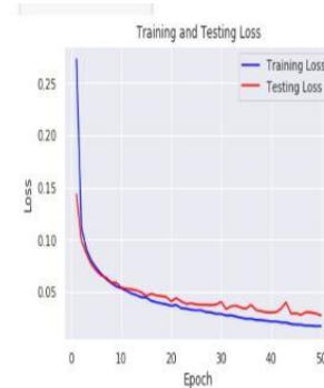
Fig. 17. Training and Testing Loss for ConvNet using Learning Rate of 0.0001 with 6 Disease Classes.
