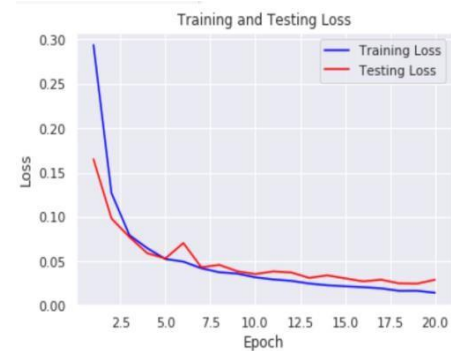
Fig. 3. Training and Testing Loss for CNN using Learning Rate of 0.0001 with 4 Disease Classes.
