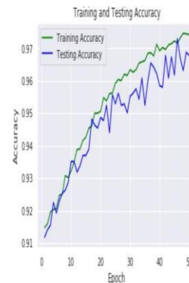
Fig. 18. Training and Testing Accuracy for ConvNet using Learning Rate of 0.001 with 6 Disease Classes.
