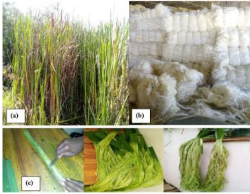
Figure 1. Natural fibres used in the study: (a) Cattail plant, (b) Sisal fibres, (c) Cattail fibre extraction process.
