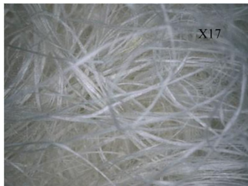
Figure 3. Micrograph of Calotropis procera bast fibres untreated taken at ×17.
