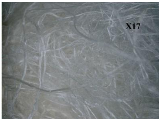
Figure 5. Micrographs of Calotropis procera bast fibres alkaline-treated taken at \times 17 .
