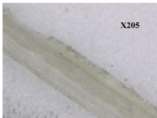
Figure 4. Micrographs of Calotropis procera bast fibres untreated taken at ×205.
