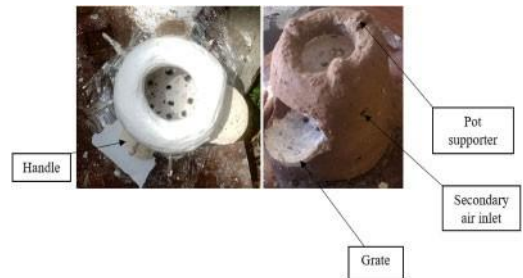
Figure 2. Stove under construction.
