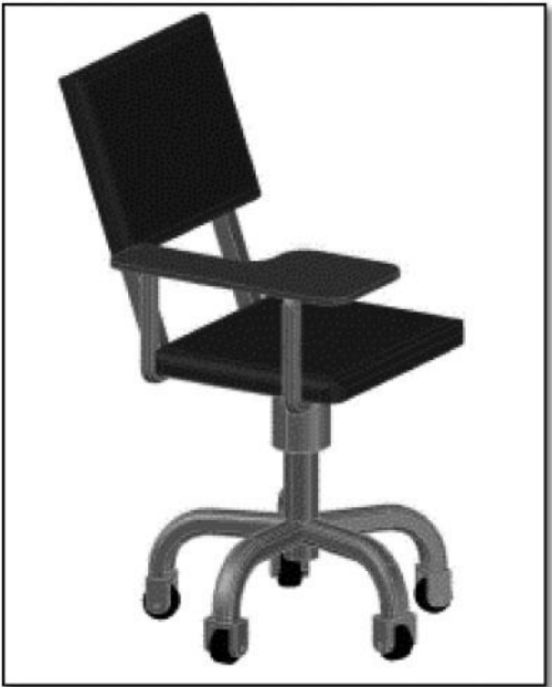
Figure 3b. Complete model of the proposed adjustable students' desktop–chair.
