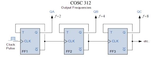
i) Explain how the above flip flop circuit works
