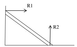
Calculate the magnitude and direction of the reactions  $R_1$  and  $R_2$  at the two ends of the ladder [8mks]
