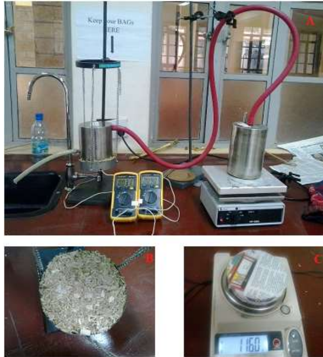
Figure 1; Experimental Set-up. A shows how the apparatus was arranged. B shows the rice husk disc and C shows the newspapers disc placed on a mass balance.
