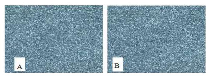
**Figure 1.** Images of RHA made using Kodak C1530 Digital Camera with 14 megapixels and 3X optical zoom. A. FRHA calcined at 700°C and in B. ORHA burnt on top of a hot metallic plate in open air.
