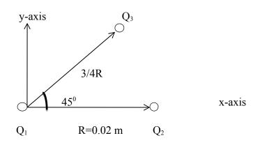
What is the net electrostatic force F1.net on particle 1 due to 2 and 3 [8mks]
