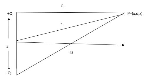
b) From the equation for potential due to a dipole at point P, show that the electric field component in the Z- direction is given by
