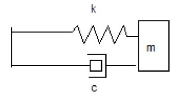
The spring is initially compressed by 20 mm.
