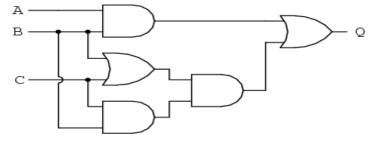
Draw the minimised product of sum of the above circuit (show the process of conversion from SOP to POS) (6 marks)
